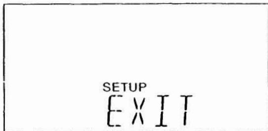
Figure 69 SETUP EXIT screen; press ACT to go back to the TIME OF DAY screen
